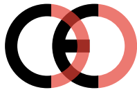
False CE Mark (too close)
